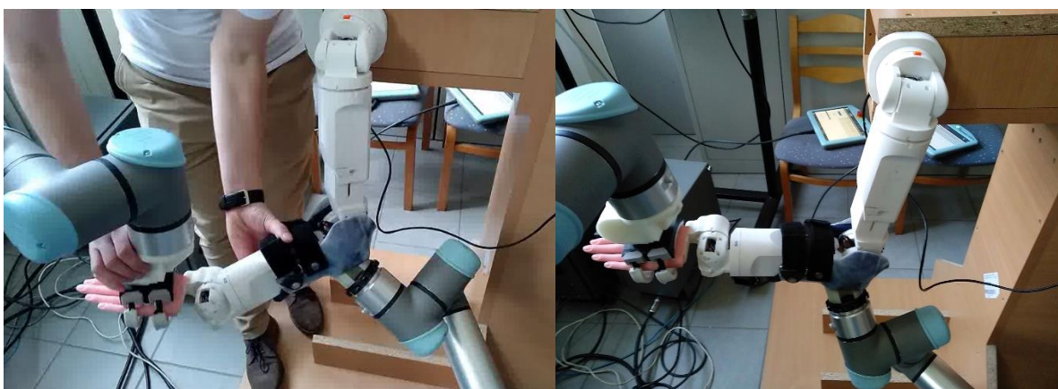
Figure 15: Safety assessment of a RACA robot. Left: the physiotherapist programs the RACA robot by hand guiding the dummy upper limb; Right: the RACA robot autonomously exercises the dummy upper limb
