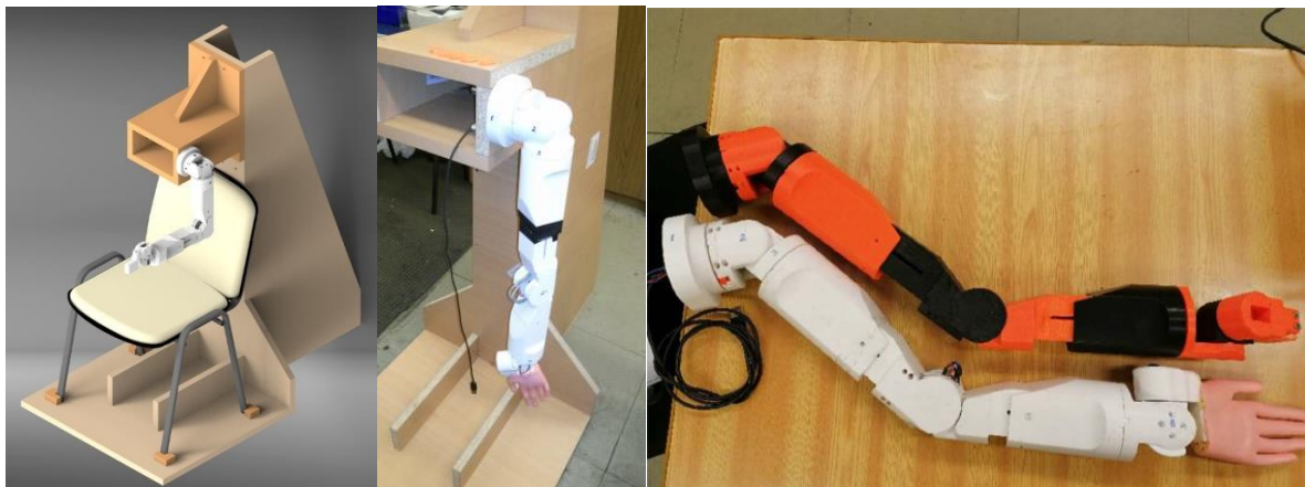
Figure 11: Left: 3D CAD rendered image of the dummy limb test rig (upper arm's length: 5%ile female, lower arm's length: 95%ile male); Middle: photo of the developed dummy limb test rig (upper arm's length: 95%ile male, lower arm's length: 5%ile female); Right: orange-black dummy limb prototype (upper arm's length: 95%ile male, lower arm's length: 95%ile male), white dummy limb prototype (upper arm's length: intermediate size, lower arm's length: intermediate size)
