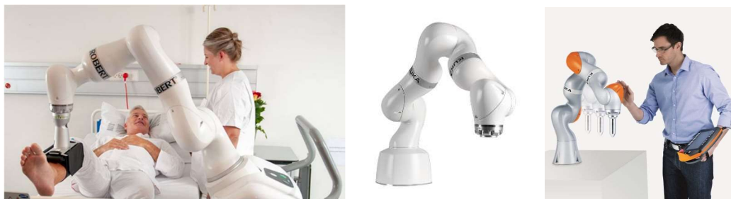
Figure 14. – The ROBERT® lower limb rehabilitation robot (left), the KUKA LBR MED medically certified cobot (centre), the KUKA LBR iiwa industrial cobot (right)
