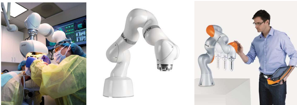
Figure 5. – Current version of the Artas iX™ robotic hair transplant system (left), the KUKA LBR MED medically certified cobot (centre), the KUKA LBR iiwa industrial cobot (right)
