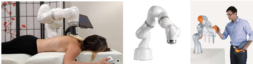
Figure 11. – The iYu Pro back and neck massaging robot (left), the KUKA LBR MED medically certified cobot (centre), the KUKA LBR iiwa industrial cobot (right)
