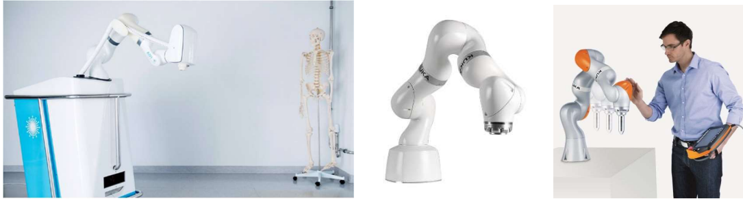
Figure 7. –The CARLO® robot-assisted cold ablation laser osteotome system (left), the KUKA LBR MED medically certified cobot (centre), the KUKA LBR iiwa industrial cobot (right)
