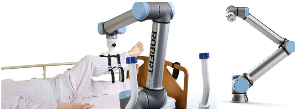
Figure 13. – First version of the ROBERT® lower limb rehabilitation robot (left), the Universal Robots UR10 industrial cobot (right)
