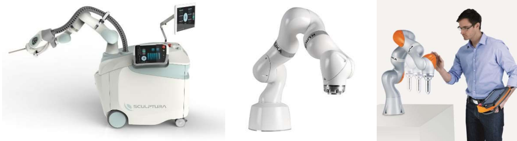
Figure 6. – The Sculptura™ directional beam image guided mobile robotic radiation therapy system (left), the KUKA LBR MED medically certified cobot (centre), the KUKA LBR iiwa industrial cobot (right)
