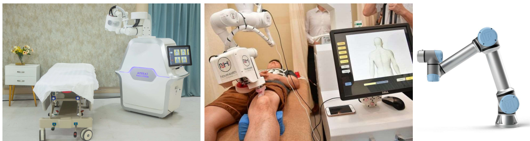
Figure 12. – The EMMA Traditional Chinese Massaging robot (left and centre), the Universal Robots UR5 industrial cobot (right)
