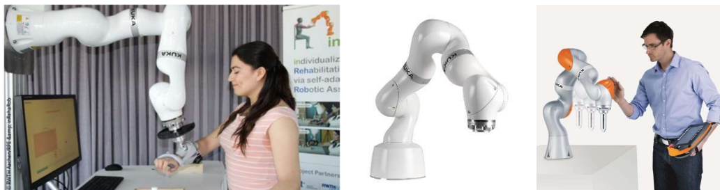
Figure 21. – The inRehaRob upper limb rehabilitation robot (left), the KUKA LBR MED medically certified cobot (centre), the KUKA LBR iiwa industrial cobot (right)
